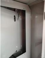
b. Remove 8 nuts, then slide the backplate down and away to remove it Nut locations: 2 on the bottom, 2 on the top, 4 on the back (top half)
