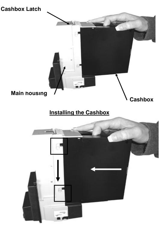
NOTE: WHEN INSTALLING THE CASHBOX MAKE SURE THE TABS ARE PUSHED FORWARD INTO THE SLOTS ON THE MAIN HOUSING AND THEN PUSH DOWN MAKING SURE THEY CLICK INTO PLACE. IF THE CASHBOX IS NOT PROPERLY INSTALLED THE BILL ACCEPTOR WILL NOT FUNCTION.
