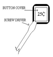
PLACE THE SCREW DRIVER AT THE EDGE OF THE BUTTON COVER AND TWIST THE DRIVER UP. REPEAT THIS FOR THE REMAINING EDGES.
