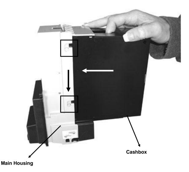
NOTE: WHEN INSTALLING THE CASHBOX MAKE SURE THE TABS ARE PUSHED FORWARD INTO THE SLOTS ON THE MAIN HOUSING AND THEN PUSH DOWN MAKING SURE THEY CLICK INTO PLACE. IF THE CASHBOX IS NOT PROPERLY INSTALLED THE BILL ACCEPTOR WILL NOT FUNCTION.
